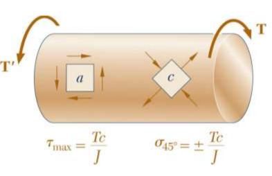
Elements with faces parallel and perpendicular to the shaft axis are subjected to shear stresses only. Normal stresses, shearing stresses or a combination of both may be found for other orientations.
