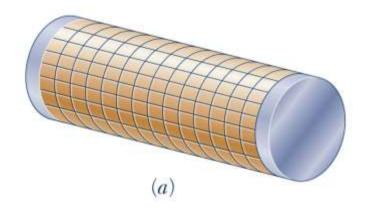
We want to make sure that the couples are applied in such a way that the ends of the shaft remain plane and undistorted. This can be accomplished by applying the couples to rigid plats, which are solidly attached to the ends of the shaft.
