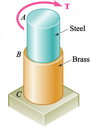
**3-17:** The solid shaft shown is formed of a brass for which the allowable shearing stress is 55 MPa. Neglecting the effect of stress concentrations, determine the smallest diameters  $d_{AB}$  and  $d_{BC}$  for which the allowable shearing stress is not exceeded.
