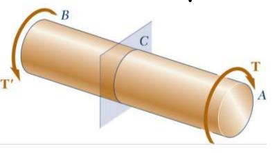
Consider a shaft subjected to equal and opposite torques at its opposite ends. The net of the internal shearing stresses is an internal torque, equal and opposite to the applied torque,
