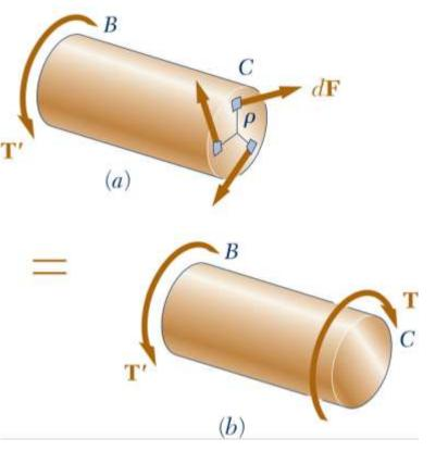
Unlike the normal stress due to axial loads, the distribution of shearing stresses due to torsional loads can't be assumed uniform.
