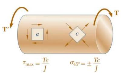
**Ductile materials** generally fail in **shear**. **Brittle materials** are weaker in **tension** than shear.
