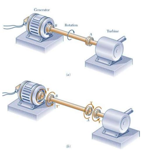
Interested in stresses and strains of circular shafts subjected to twisting couples or **torques**
